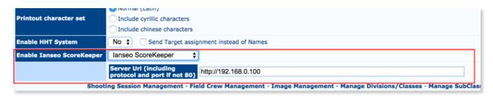
The server url is the ip-address that was assigned by the wireless router. Enter "http://" together with the ip-address and choose Normal to enable the app settings. *Note:* if this value of the ip-address changes for any reason, the value here must be updated accordingly.
