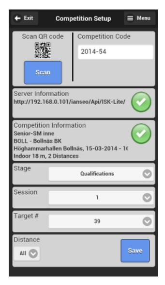
It is possible to configure the app manually by pressing the Menu button in the upper right corner and choosing *Manual Entry* instead of scanning the QR code. This will allow manual entry of the url and the competition code. Note that manual entry of the url will require technical knowledge of the IANSEO computer installation and setup.
